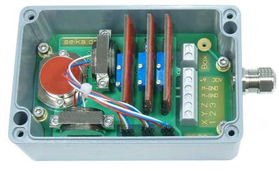
Sensor box containing three SEIKA sensors and three signal conditioners with 0...5V or +/-4V output.
